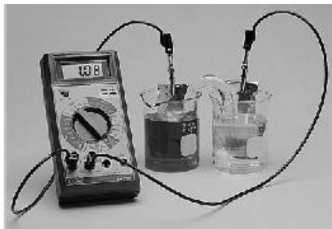
A zinc-copper voltaic cell
